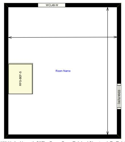
Get The Overall Width And Length Of The Room From Finished Sheetrock To Finished Sheetrock
