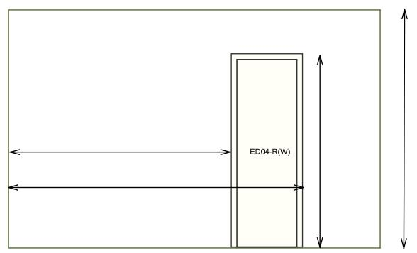
Measure From The Corner To The Edge Of The Moulding From The Same Corner, Measure To The Other Side Of The Moulding Measure The Ceiling Height
