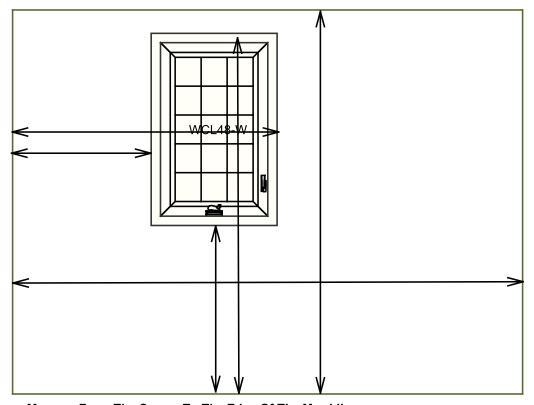
Measure From The Corner To The Edge Of The Moulding
