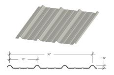
Applications: Roof and Wall Coverage Width: 36" Rib Spacing: 12" on Center
