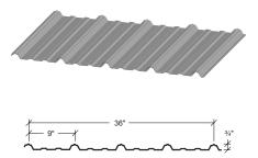
Applications: Roof and Wall Coverage Widths: 36" Rib Spacing: 9" on center Rib Height: 3/4"
