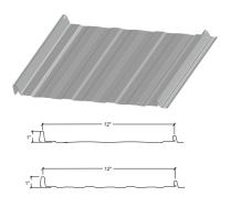
Applications: Roof Coverage Widths: 16" Rib Height: 1" Minimum Slope: 3:12
